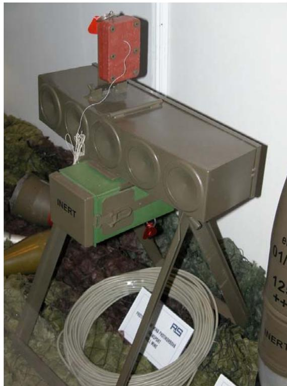
The Horizont displayed in a victim-activated, anti-personnel mode, with tripwire and a sensor contact cable fusing system
